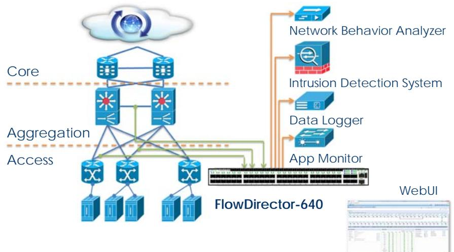
The FlowDirector can help network administrators to manage monitoring network without service interruption. Also it helps network administrator load balance the traffic across multiple monitoring devices to provide the analytical processing power to where it is critically needed.
