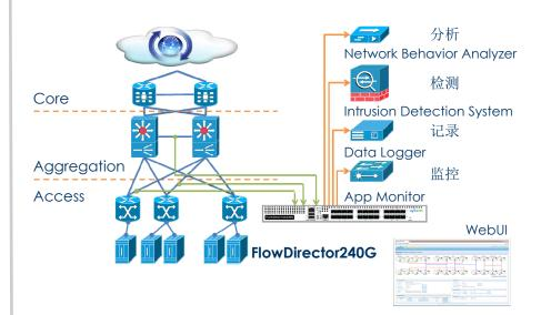
FlowDirector can help network administrators to manage monitoring network without service interruption. Also it helps network administrator load balance the traffic across multiple monitoring devices to provide the analytical processing power to where it is critically needed.
